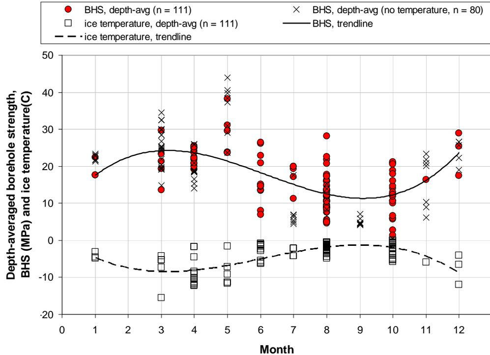
Figure 1 Depth-averages of borehole strength (BHS, circles & crosses) and ice temperature (squares) for individual boreholes, after [1]
