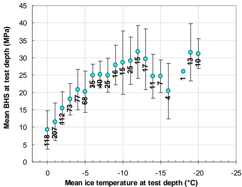
Figure 4 Mean and st. dev. of old ice borehole strength (BHS), binned by ice temperature, after [1]
