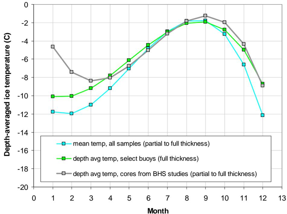
Figure 3 Comparison of results from three approaches for obtaining bulk ice temperatures
